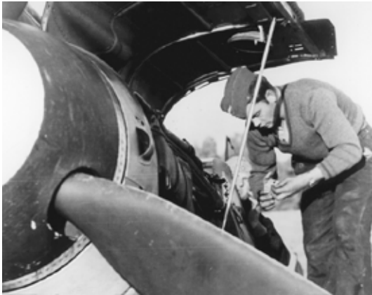
A mechanic labors over the Daimler-Benz engine of this Bf 109. Courtesy National Air & Space Museum, Smithsonian Institution
