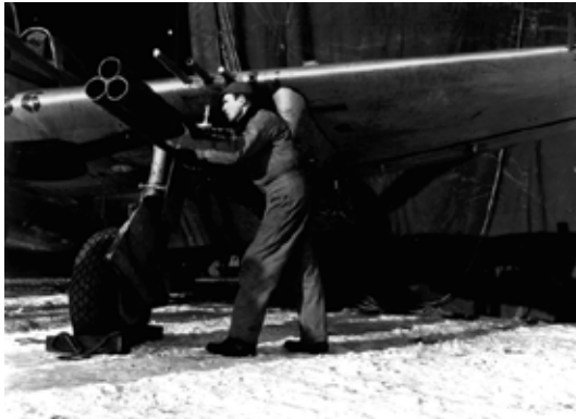
Bazooka rocket tubes employed by the USAAF, slung under the wing of a P-47. Courtesy National Air & Space Museum, Smithsonian Institution
