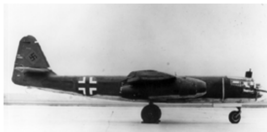
The Arado 234. Note the periscope on top of the canopy. It was a modified tank periscope used by the pilots to check their tails and drop their bombs. Courtesy National Air & Space Museum, Smithsonian Institution
