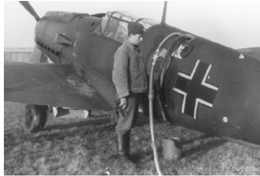
A mechanic refuels a Messerschmitt 109. Courtesy National Air & Space Museum, Smithsonian Institution
